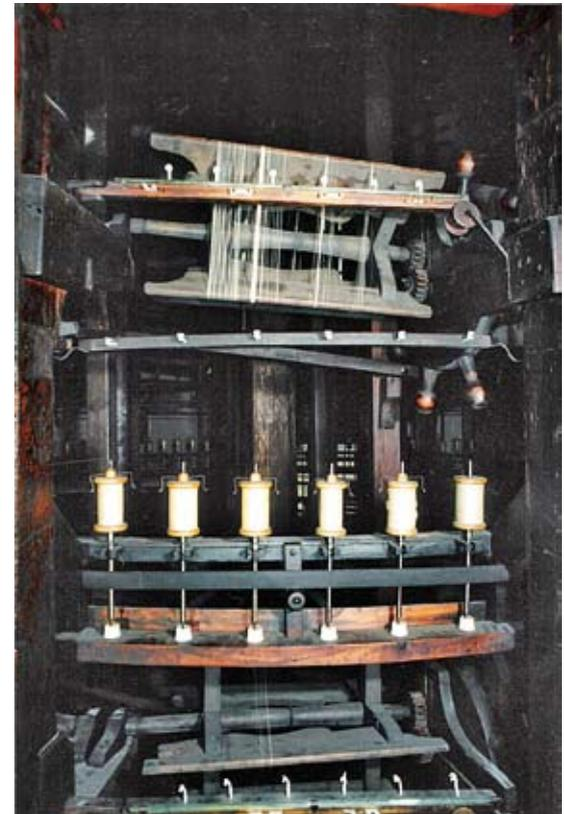
Machine for winding onto spools.
