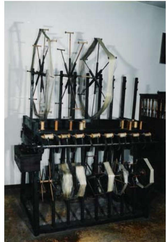
Machine for winding onto spools.
